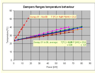
RF power level vs temperature. Courtesy F. Perez
