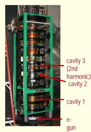
SLS klystron (EEV K3418P) Courtesy L. Stingelin
