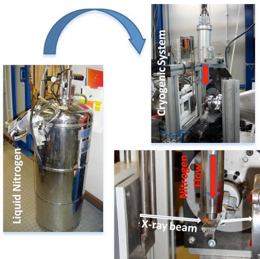
Figure 1. Illustration of the set-up combining synchrotron SAXS with a cryogenic system.
