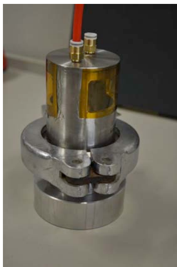
Figure 1. Sample cell used to suppress radiation damage of the samples during the X-ray measurements. The cell is equipped with entry and exit kapton windows and the gas inlets and outlets allow to keep the sample under nitrogen atmosphere.
