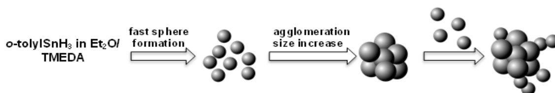
Scheme 2. Schematic growth process of the Aryl@Sn (Aryl= o -tolylSnH 3 ) in Et 2 O
